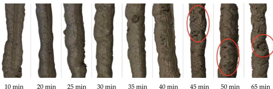
Figure 6. Quality of the single-layer extrusion: observation of the fluid consistency of extrusion from 10 min after mixing and crack occurrences from 45 min after mixing.
