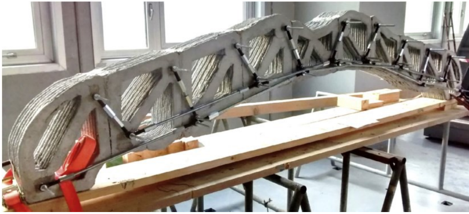
Figure. 2-12 System of outer geometry reinforcement beam [31].
