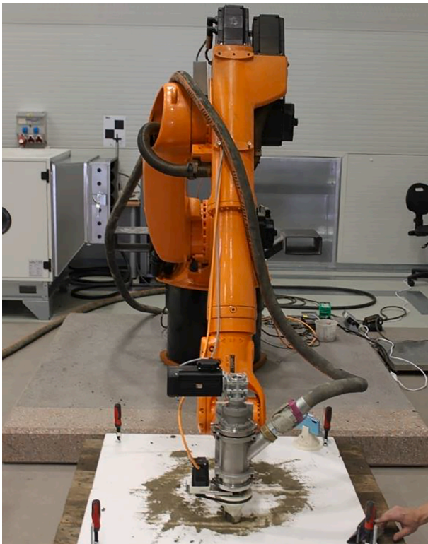
Fig. 1. Hose routing issues in the robotic arm.
